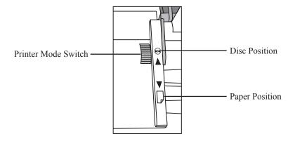
1. Move Printer Mode Switch to paper position.
